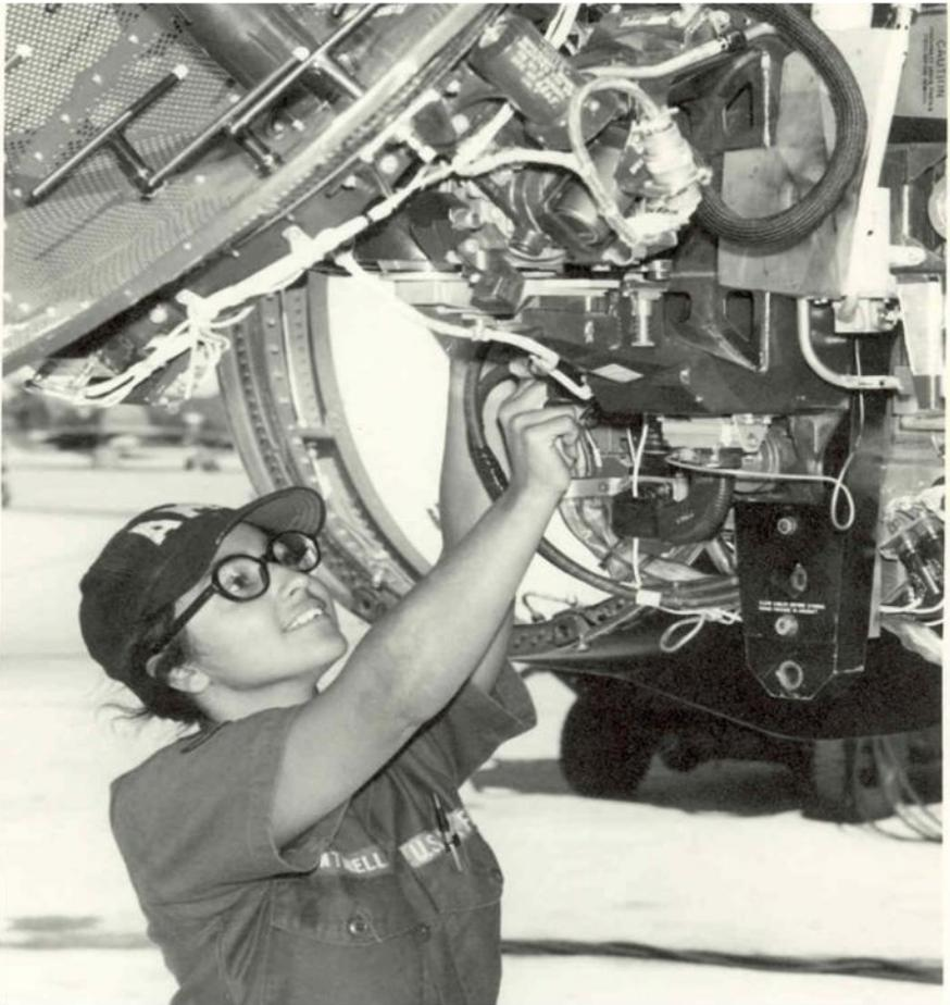
**A 35th Avionics Maintenance Squadron Airman inspects an F-4 Radome on the flight line at George AFB, California in 1975.**
